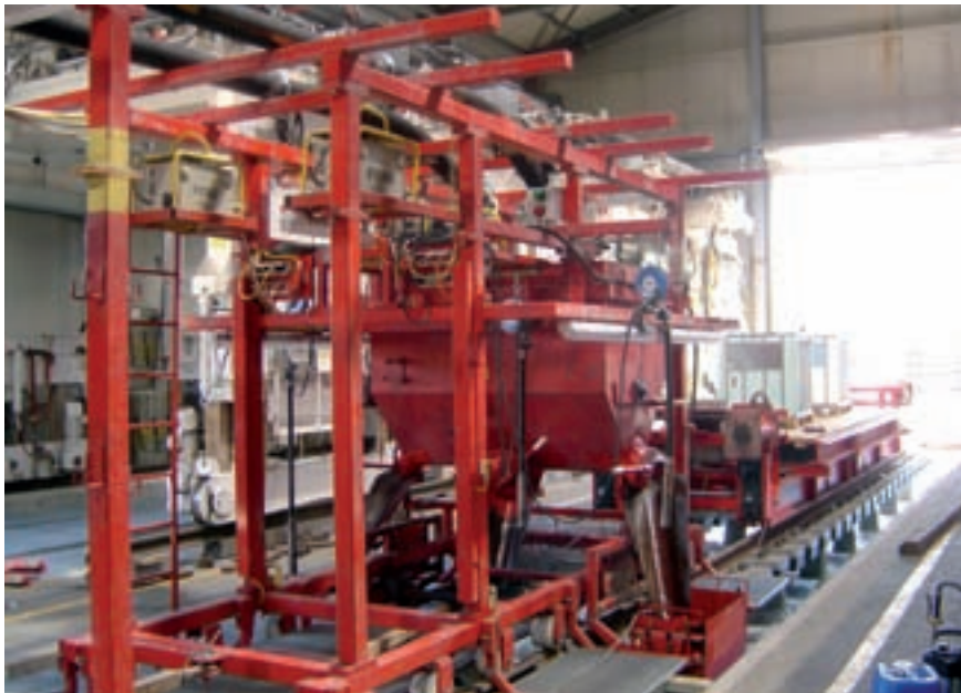
The patented paving machine on its own railcar.
