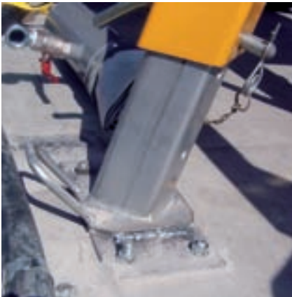
The concrete pump is screwed to the superstructure of the railcar
