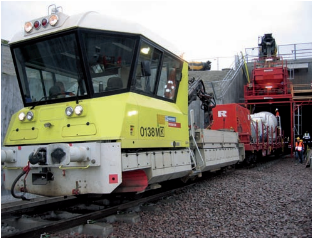
A locomotive with the rail wagon shuttles between the concrete handover point and the concreting train
