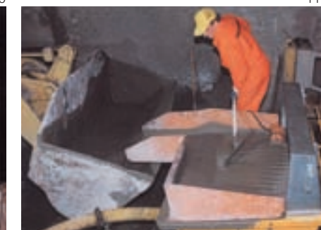
Draining the residual material by reverse pumping into a mechanical shovel for distribution in cavities
