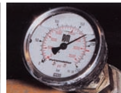
Maximum pressure in the concrete: 185 bar
