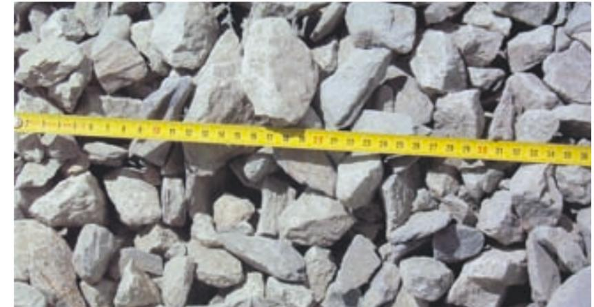
Aggregates with 50 mm maximum particle size are simply expected of the Putzmeister M 36 concrete pump (boom delivery line 125 mm)
