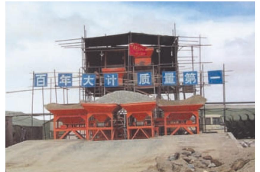
A concrete mixing station along the line with a capacity of 2 x 50 m³/h. One of the biggest problems when constructing the Tibet railway is the lack of water.
