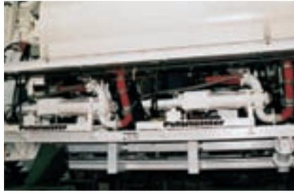
Mortar injection pumps ergonomically positioned on the trailing axle of the tunnelling machine
