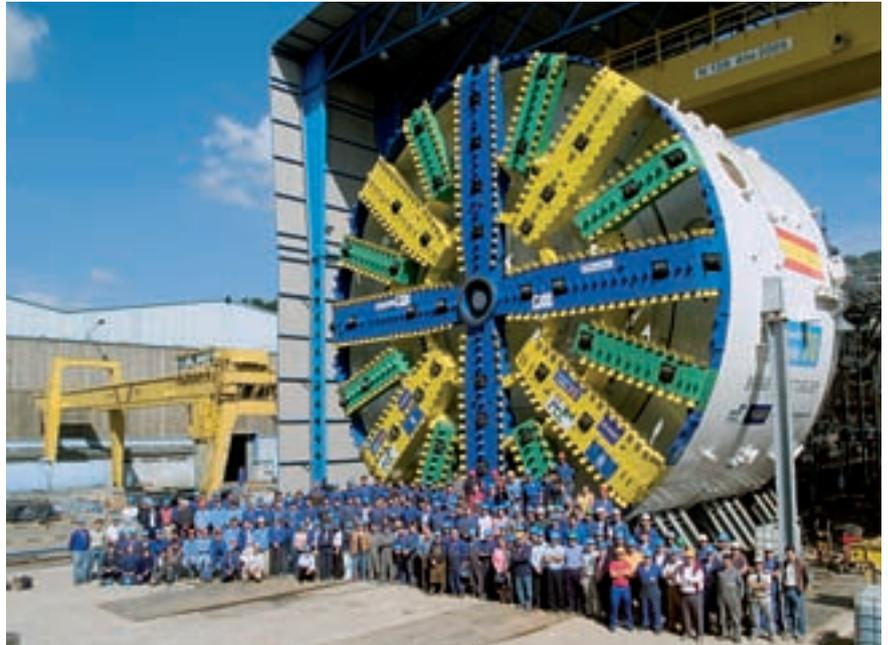
The tunnelling machines for the M30 motorway tunnel have a diameter of over 15 m. Pictured is the tunnelling machine supplied by Mitsubishi Heavy Industries (Photo: MHI / Duro Felguera)
